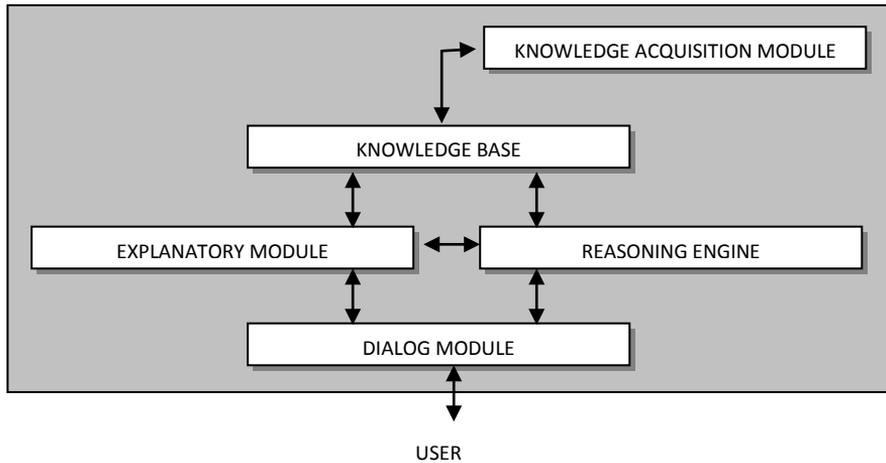
**Fig. 1 Architecture of a typical expert system (Mulawka, 1996)**
